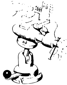
FIG. 43. The Hobby Vise, used by model makers and kindred folks, has a clamping arrangement in its base that allows it to be tilted in practically any direction and then firmly locked in place.
