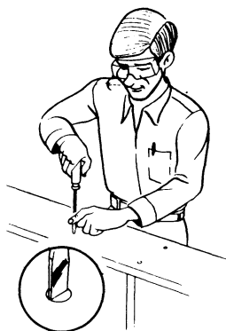
FIG. 7. Cal is using the right technique in driving this screw home. The blade of the screwdriver is a snug fit in the slot of the screw and does not quite project to the edge.
