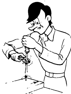
FIG. 12. Special screwdriver bit that can be chucked into a carpenter's brace.
